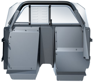
Setina PK1186ITU20-TM 10XL C2 Partition, Recessed, C Poly Sliding window, Tall Man Installation Kit
