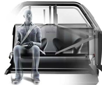
Center pull seat belts allow officer to buckle seat belt from outboard position to prevent leaning over occupants
