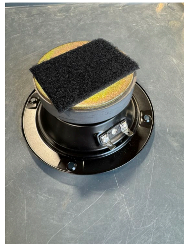
Step 5: Apply fuzzy side Velcro to back of speaker. (prevents rattles on roof)
