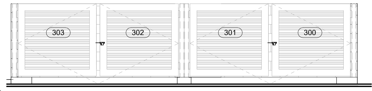
41 TRASH ENCLOSURE FRONT ELEVATION 1/4" = 1'-0" RE: CITY OF EXETER IMPROVEMENT STANDARD SHEET M-6
