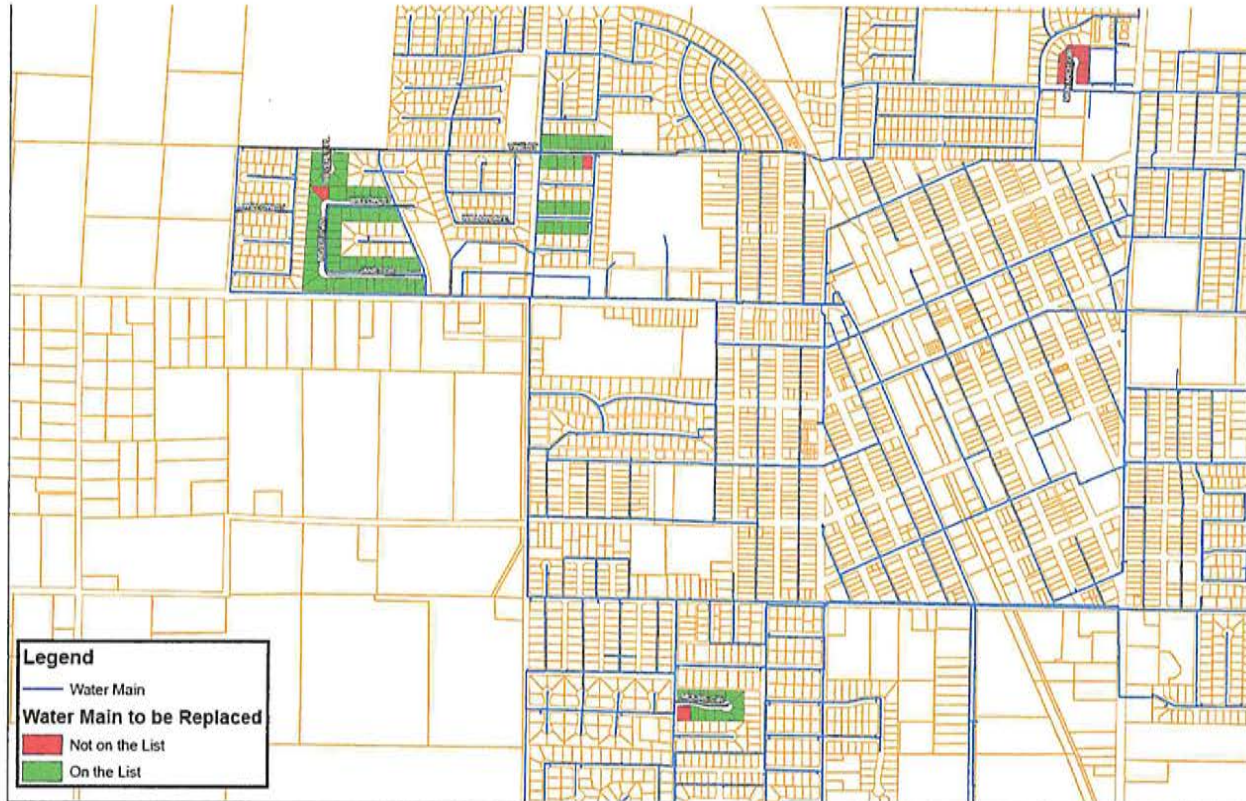
Map 1 Frequent Water Leak Streets
